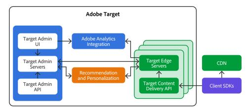
Figure 1: Adobe Target Solution Architecture
